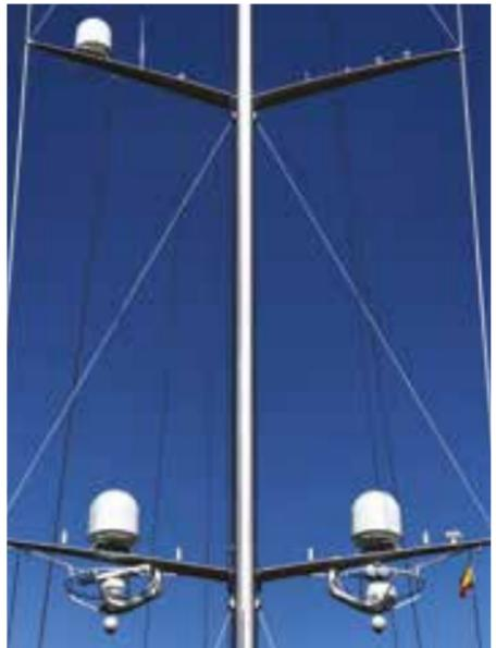
Previously, the yacht was fitted with a matching pair of very large Ku-band SeaTel 4012 domes, with a combined weight of just under 300kg. To reduce the weight and windage of the hardware installed, and improve the physical appearance of the yacht’s rig, the decision was made to opt for Fleet Xpress to enable high-speed connectivity and global streaming IPTV [internet protocol television] solution.
