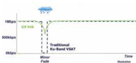
Adaptive Coding and Modulation (fwd link) and A-TDMA (rtn link) used in GX network enables the system to assign more power or to gracefully slow throughput to avoid link loss
