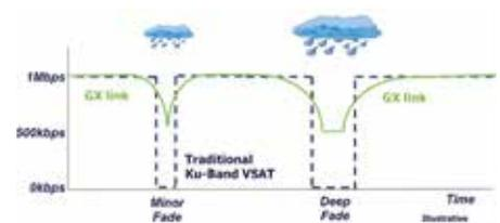
Use of the NSD and L-Band back-up can avoid complete loss of link
