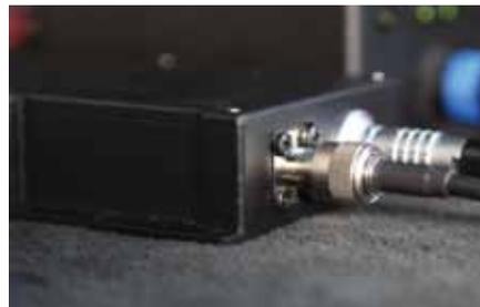
**SlingShot™** – Spectra's small, lightweight external appliqué for military radios, allows low-latency voice and data regional communications with the additional option of connecting to an out-of-theatre rear based command node
