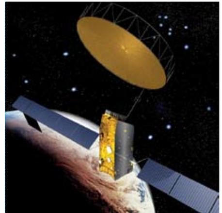
Each Inmarsat-4 is 60 times more powerful than an Inmarsat-3 satellite and has highly sophisticated spot-beam configuration capability
