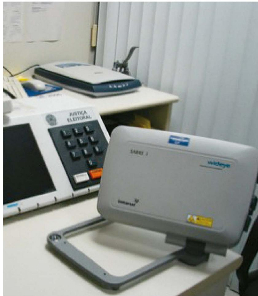
The BGAN terminals offered flexible service options, including simultaneous voice and data connectivity at speeds up to 492 kbps—about 50 times faster than the previous service. Addvalue's Wideye SABRE 1 terminal was compact, robust, simple to use, and inexpensive. Value added services—including bulk activations, data encryption, dedicated VPN, terminal authorization, cost controls, and real-time traffic monitoring—proved essential to success.
