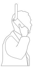
Stand outside with a clear view of the sky with the phone antenna pointing upwards. There must be a clear line of sight between the phone's antenna and the satellite.
