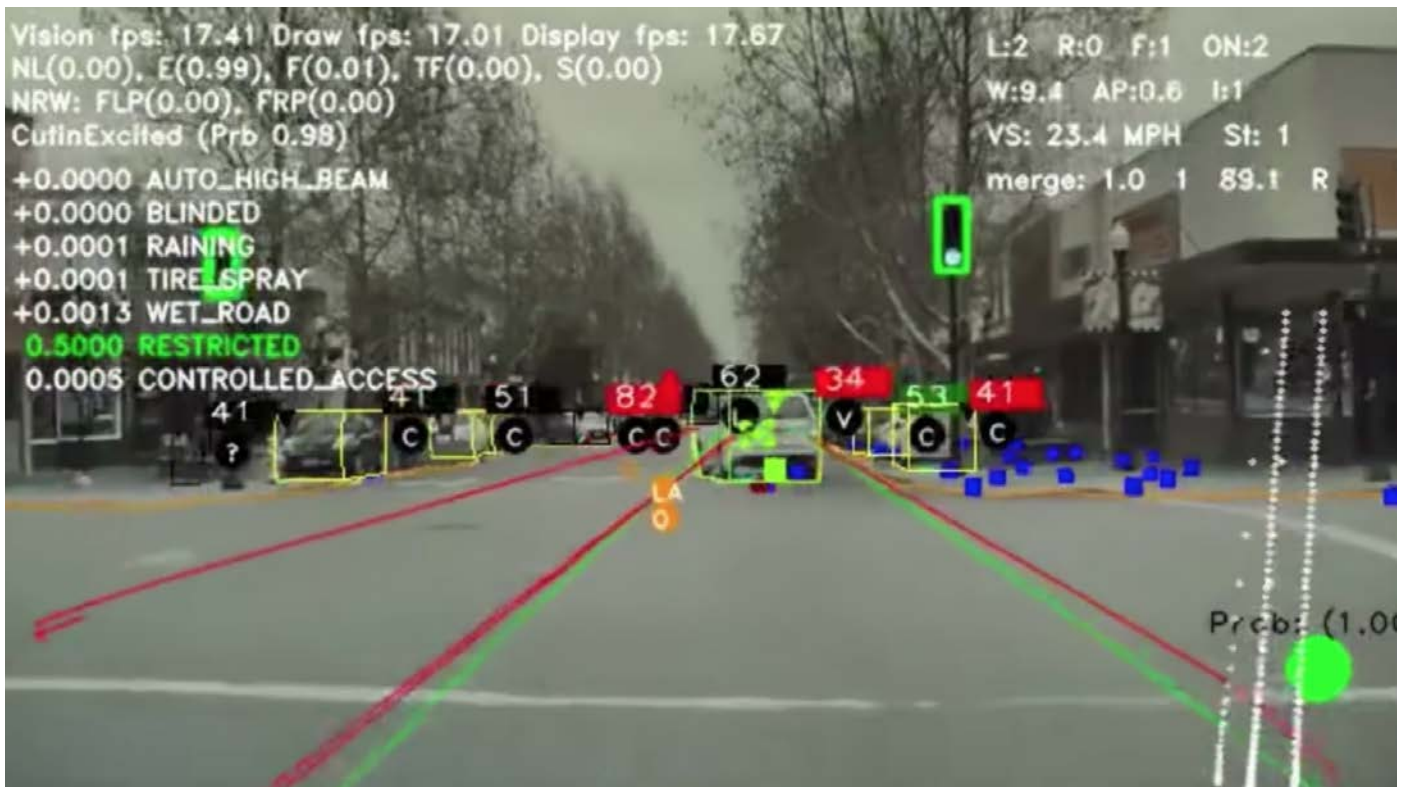
Figure 12 Tesla's autopilot system at work. The system perceives real-world objects using machine vision and then classifies them (e.g. car, stop sign, etc.) using machine learning. 33
